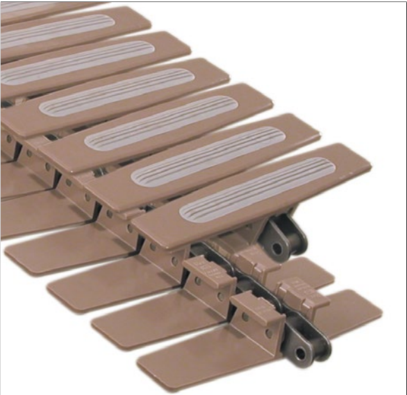
Photo shows 1873 TAB SuperGrip TableTop Chain with High Friction Inserts and top plates molded in Low Friction (LF) material on Carbon Steel (S) base chain.
